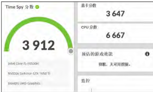
▲3Dmark显卡基准测试,2K分辨率的Time Spy DX12场景,Z3 Air的GTX 1650Ti独显成绩是3647,略高于GTX 1650的3533
